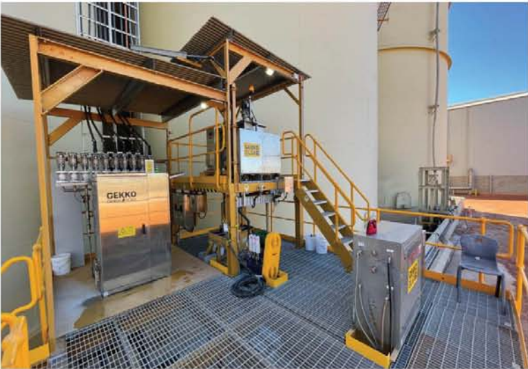
The Carbon Scout (left) and the Gekko OLGA (right) at Gruyere Mine in Western Australia. The combination of OLGA (OnLine Gold Analyser) and Carbon Scout, supported by the Gekko Sample Delivery System means all CIL/CIP sampling can be done conveniently and safely at ground level.
